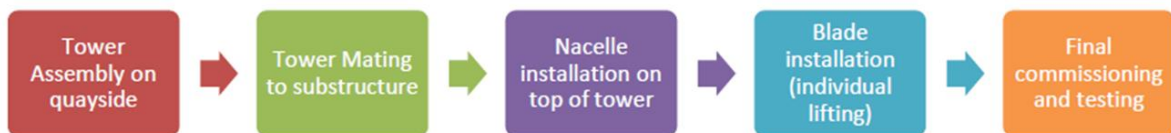
Figure 2.2 Moneypoint Hub WTG Staging process (Source: ESB, 2023)
